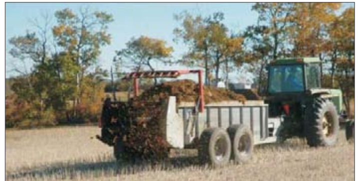
(Left) The LEON Vertical Silver Spreader transporting manure from a feedlot and (right) the LEON Horizontal Silver Spreader transporting manure to a fall field in preparation for next years planting year. Units under went months of intense testing on a Saskatchewan feedlot.
