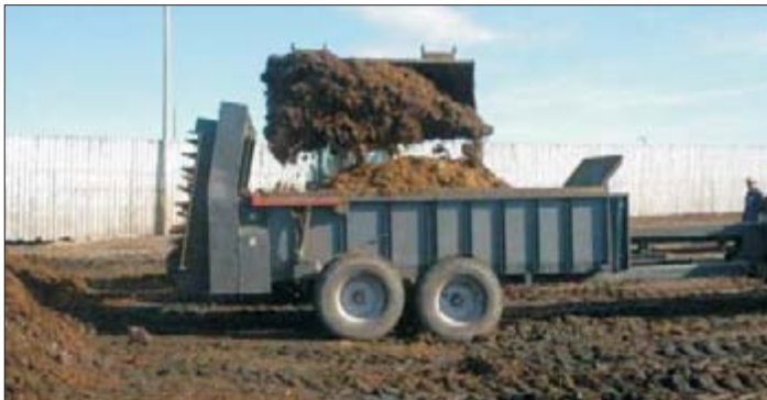
(Left) The LEON Vertical Silver Spreader transporting manure from a feedlot and (right) the LEON Horizontal Silver Spreader transporting manure to a fall field in preparation for next years planting year. Units under went months of intense testing on a Saskatchewan feedlot.
